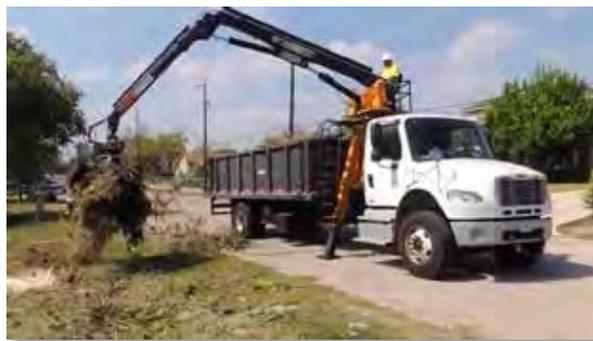
Figure 3-4. Knuckle Boom Truck
