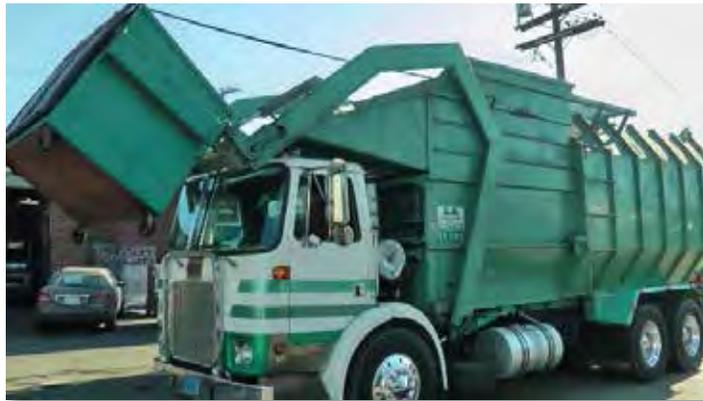
Figure 3-2. Commercial Front Load Truck
